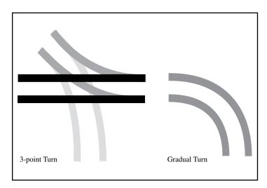
To help maximize the life of a multi terrain loader undercarriage, counter rotations should be used only when required, such as in very confined areas. Instead, use more gradual turns while slowly moving forward or in reverse.
