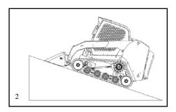
Turning when on a slope is an operation that requires special attention. When turning to go DOWN a slope, first stop the machine. Then slowly turn the machine while backing down the slope (Illus. 3). When turning to go UP a hill, stop the machine, and turn while you slowly back down the slope or until the machine is facing the desired direction of travel. Then carefully proceed forward.
