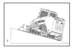
Avoid making direct 90-degree turns when operating on a slope-either on a side hill or straight up and down. Sharp turns on slopes cause unnecessary wear on track lugs and can shove material between the track and roller wheels. In some cases, this could lead to track derailment and track damage.
