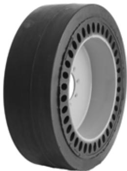
This tire has the same advantage as the regular Flexport tire with a smooth tread for special applications where traction is not an issue. Flexport smooth tread tires are suggested for work environments such as scrap and glass because these materials provide traction and can cause chunking of a construction type tread. The smooth tread design alleviates this type of wear damage.
