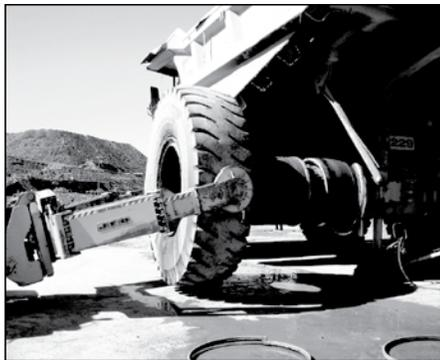
The QCR System is designed to improve mine site productivity, minimize downtime associated with tire servicing and to improve safety for tire service personnel when changing tires on large mining trucks. Compared to the standard fitment five-piece rims currently offered, the QCR System provides an increased crack test interval, longer rim life, improved safety and fewer rim based remove/install procedures during tire changes.
