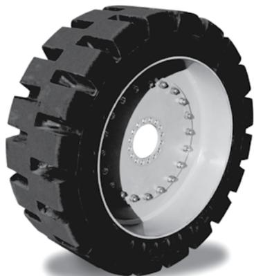
This solid tire runs on unimproved surfaces with an improved ride without sacrificing the strength of a solid. Its innovative design features Flexport, a series of holes mold- ed through the outer ring of the side wall. These ports result in greater tire flexibility for a more cushioned ride than solid tires. They also serve as a means of absorbing shock that would have otherwise been transferred to the machine and the operator.
