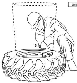
The trajectory path may be the gravest area of danger if a tire bead ruptures and/or a tire violently explodes due to misapplication, improper inflation, overloading, or for any other possible reason.
