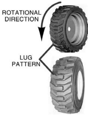
Cat pneumatic skid steer tires are directional tires. The lug or “tread” pattern is designed to enhance traction. By specifying the rotational direction of a tire, cross ribs and grooves are laid out so that traction improves in slippery applications. When ordering a tire and wheel assembly, it is critical to know on which side the tire will be mounted. If an incorrect tire is specified, it will need to be remounted in the correct direction of rotation.
