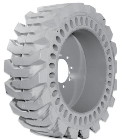
NOTE: A 31 x 6 x 10 solid tire replaces a 10 x 16.5 pneumatic tire and a 33 x 6 x 11 solid tire replaces a 12 x 16.5 pneumatic tire.
