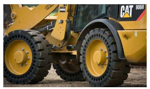
Cat Flexport Tires for Compact Wheel Loaders are a 1-piece tire / rim design and are available in directional construction, smooth and OTR tread patterns.
