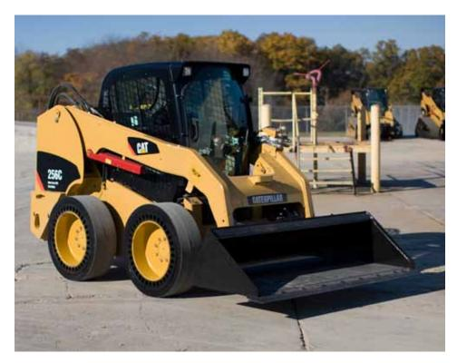
Cat Flexport Tires for Skid Steer Loaders are a 1-piece tire / rim design and are available in directional construction, smooth and OTR tread patterns.
