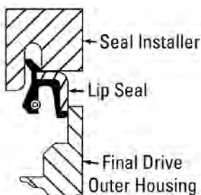
Cross section of installer showing shoulder and counterbore
