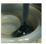
Cat Filters eliminate the potential for gaps by inserting the filter media directly into the end caps as they are formed.
