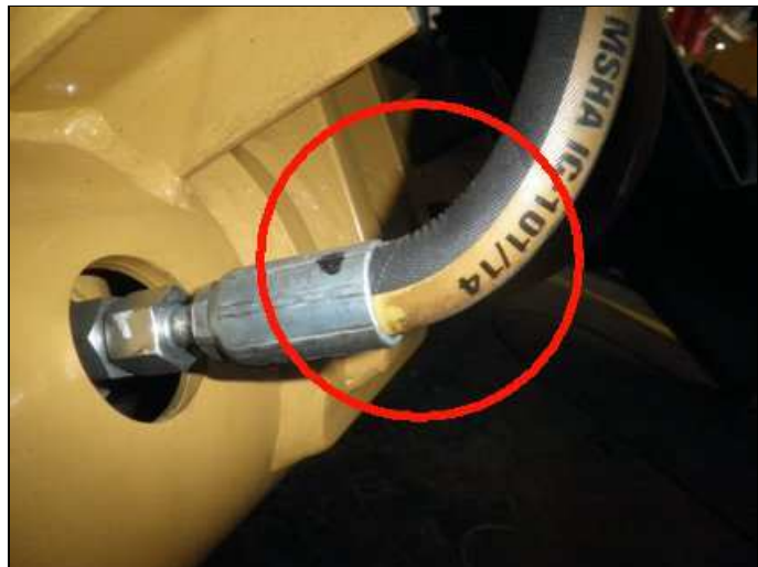
Figure 2: Hose bent at coupling.
