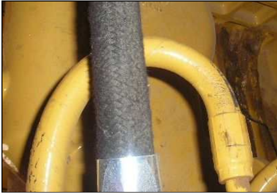
Figure 3: Hose exceeds bend radius (yellow hose).
