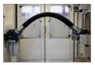
To simulate punishing conditions, Caterpillar impulse-tests hose assemblies at 130% of operating pressure for one million cycles double the SAE standard of 500,000 cycles.
