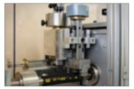
The number one cause of hose failure is abrasion. Cat ToughGuard hose, designed for severe abrasion applications, features a polyethylene cover that has surpassed two million cycles of abrasion testing without failure. The SAE standard is 39,000 cycles.
