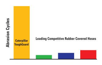
\* The International Standards Organization (ISO) abrasion resistance test requires a 50N (11 lb) steel tool to be cycled back and forth along the length of the hose until the cover wears away to the point of wire exposure.
