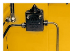
The flood and safety valve.
