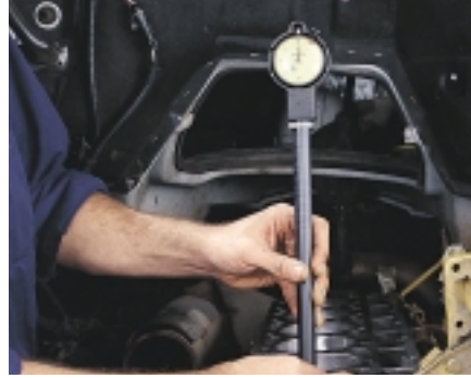
Inspect the parent bore.
