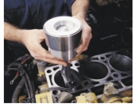
Use the installation tool to install the Reman Piston Pack quickly and easily.
