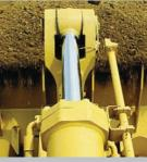
All Reman Rods are straightened, ground, chrome plated and polished; or they are replaced (re-rodded), depending on the extent of wear or damage. All re-rods are induction hardened, improving resistance to nicks and dents to extend seal life. Most feature inertia-welded eyes for superior strength. All new bearings are installed and eyes replaced with Cat parts if needed.
