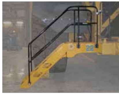
Cat powered access systems for other Cat trucks mount at bumper level.
