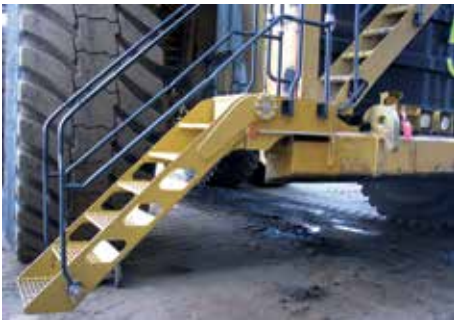
797-797B powered access system (442-1749) mounts to top of bumper for extra damage resistance in soft underfoot conditions.
