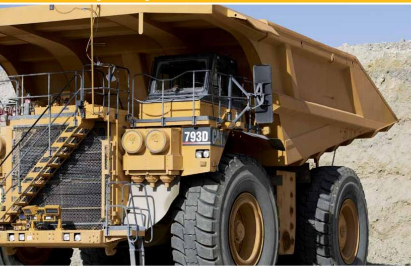
Caterpillar is pleased to announce the availability of a Front wheel cover with sight glass retrofit kit for many Large Mining Truck models. The sight glass improves serviceability, by providing visual access to bearing oil level and reducing front wheel oil level inspection time. Wheel covers without sight glasses require removal of the drain plug to check oil level.
