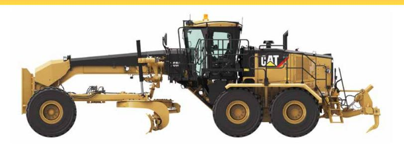
Caterpillar introduces an access platform field retrofit package for the 16M Motor Grader. This optional system provides a wraparound platform with rear enclosure walkways, left walkway lighting, rear fenders, primary left rear foldable ladder, and right front secondary egress ladder. The retrofit package provides a safe and sturdy platform for operator access, machine servicing and window cleaning.
