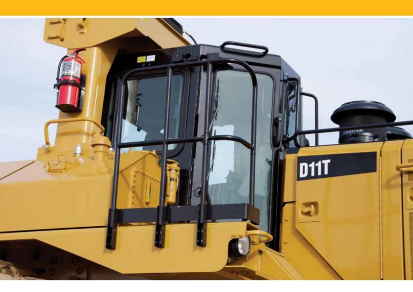
Caterpillar is pleased to announce the availability of a Guardrail retrofit kit for many D10 and D11 Track-Type Tractor models. Heavy-duty fender guardrails are strategically placed to aid operators getting on and off the machine and provide safer access to service points located on the left and right fenders.
