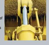
All Reman Rods are straightened, ground, chrome plated and polished; or they are replaced (re-rodded), depending on the extent of wear or damage. All re-rods are induction hardened, improving resistance to nicks and dents to extend seal life. Most feature inertia-welded eyes for superior strength. All new bearings are installed and eyes replaced with Cat parts if needed.
