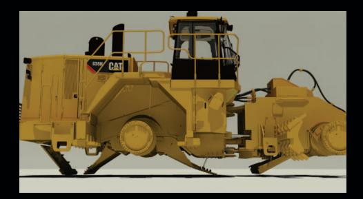
While the previous design required two service technicians, only one is now needed. Most of the bolts have been moved topside to reduce wear and closer to the outside of the machine for easier access and reduced service time. Many of the guards are now hinged internally to eliminate catch points. The front and rear axles now have guarding and rear trunnions are completely closed. The rear bumper guard and engine end frame guard are hydraulically actuated for easier raising and lowering.
