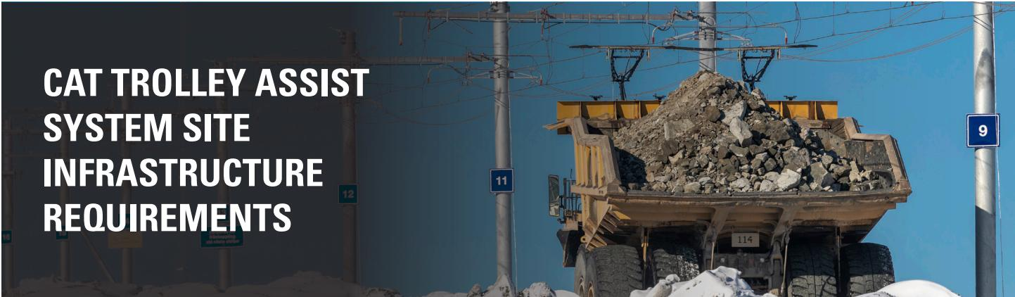
The Cat Trolley Assist System requires incremental truck iron and significant site infrastructure footprint to enable its operation. There are five key elements of the site infrastructure, they are: AC substation, DC substation(s), support poles, catenary lines, and the load height check. Site infrastructure for the trolley system must be provided by a third-party.
