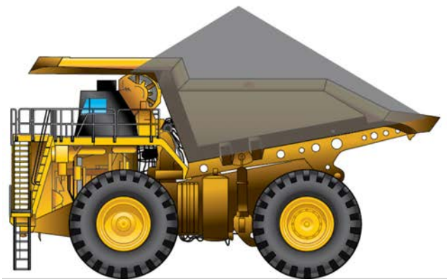
CORRECT LOAD PLACEMENT
