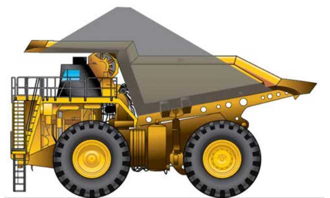
INCORRECT LOAD PLACEMENT
