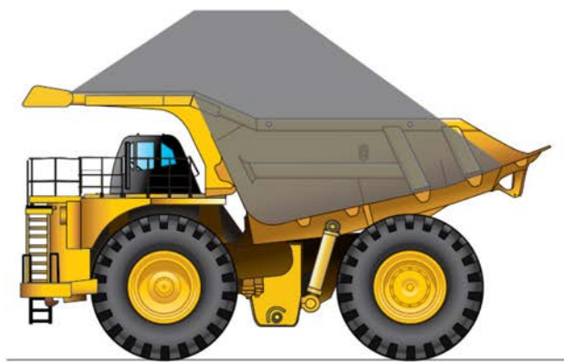
INCORRECT LOAD PLACEMENT
