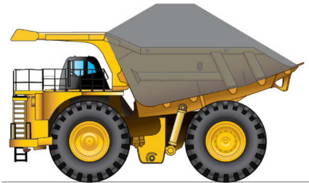
CORRECT PAYLOAD PLACEMENT
