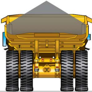
CORRECT LOAD PLACEMENT
