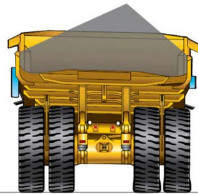
INCORRECT LOAD PLACEMENT
