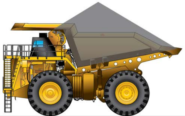
CORRECT PAYLOAD PLACEMENT
