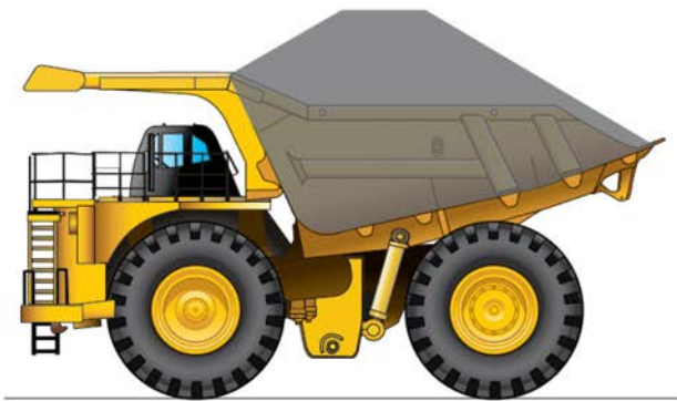
CORRECT LOAD PLACEMENT
