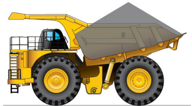
INCORRECT PAYLOAD PLACEMENT
