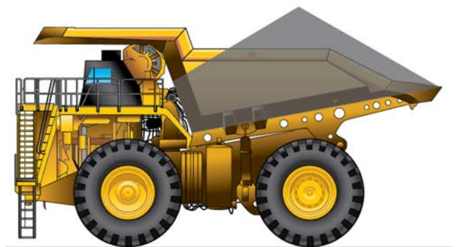
INCORRECT PAYLOAD PLACEMENT
