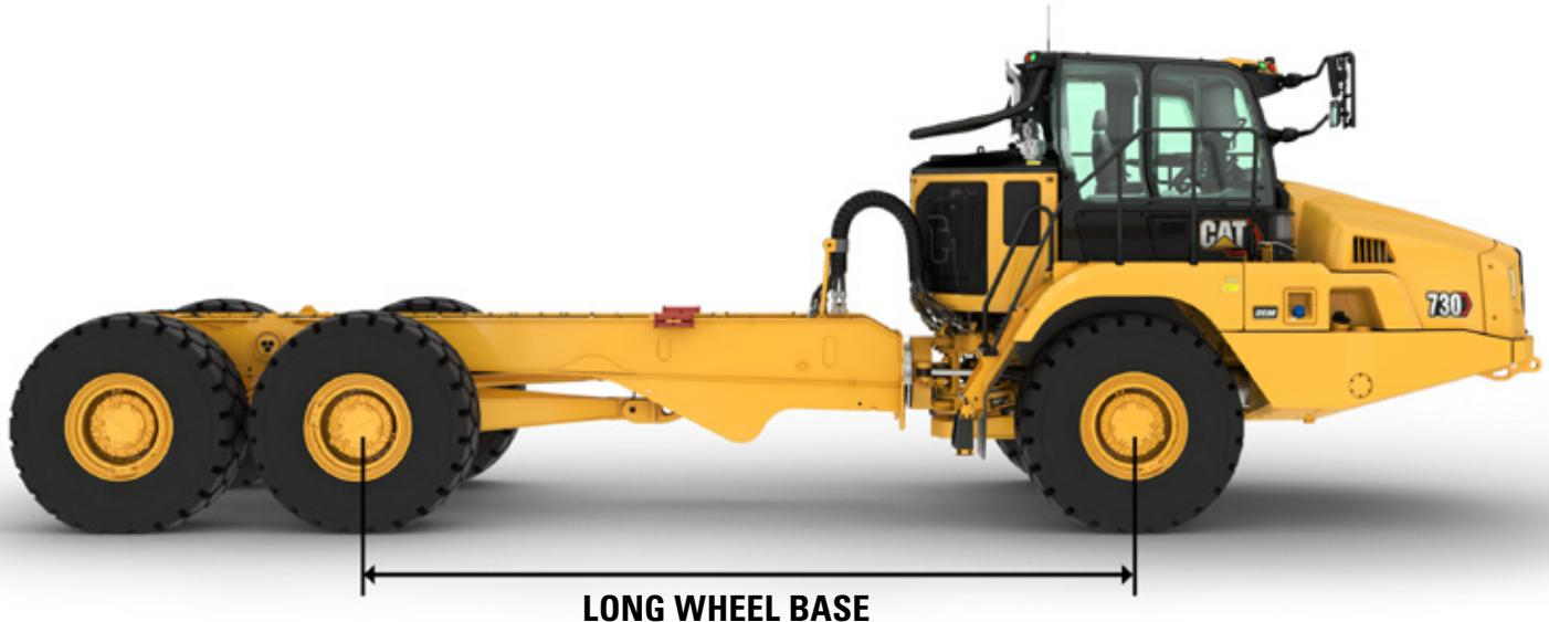
While the Bare Chassis in the long wheel base with hoist cylinders configuration is not offered as a factory option, hoist cylinders can be ordered separately for OEM / customer installation. Please contact OEM Solutions for more information.
