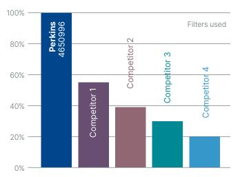
Injectors protected with Perkins filters exhibited noticeably less wear and fuel leakage when compared to the injectors tested with the competitive filters.
