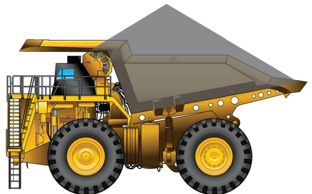
CORRECT PAYLOAD PLACEMENT
