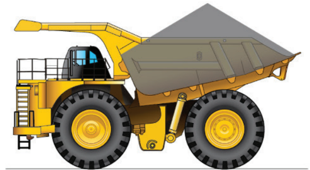
INCORRECT PAYLOAD PLACEMENT
