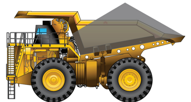
INCORRECT PAYLOAD PLACEMENT
