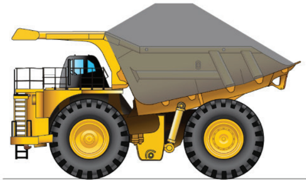
CORRECT PAYLOAD PLACEMENT
