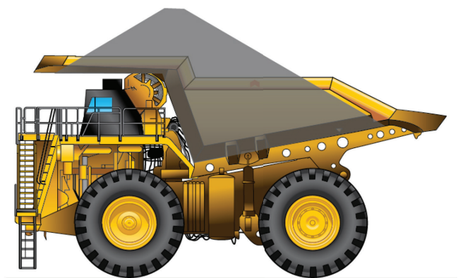
INCORRECT LOAD PLACEMENT
